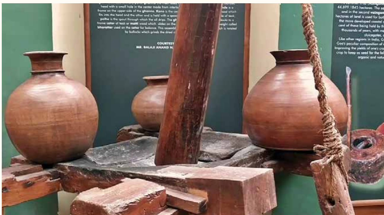
The part of the ghano wherein coconuts can be crushed to obtain oil (Photo: Srilaxmi)
